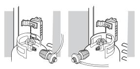
Note: This connection tightens clockwise and will not allow gas to flow unless the connection is tight. The connection requires tightening by hand only
